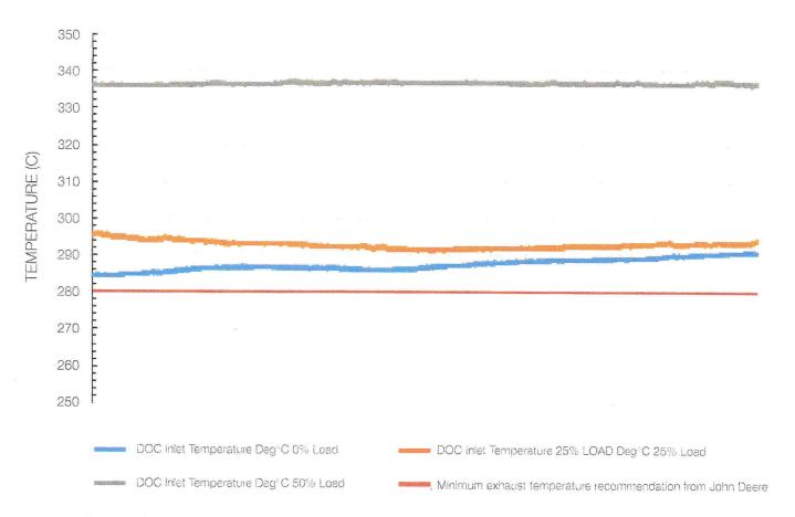
Test results show that engine exhaust temperature remained above the minimum recommended temperature threshold, regardless of load.
