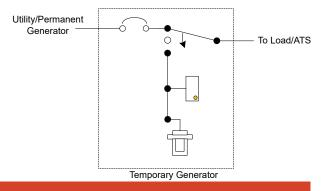
Service entrance rated TMTS with 3 position rotary to transfer between utility and temporary source
