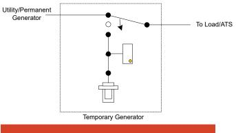
Base TMTS with 3 position rotary to transfer between permanent and temporary source
