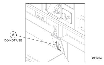
Figure 3-19. NOT Lifting Points (Four Locations)
