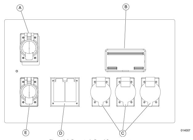
Figure 2-6. Receptacle Panel Components
