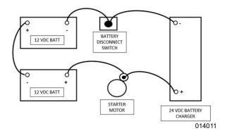
Figure 3-1. Connecting Battery Charger
