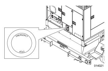
Figure 3-16. Emergency Stop Switch
