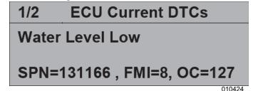
Figure 2-15. ECU DTC Page—Current DTCs
