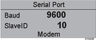
Figure 2-17. Serial Port Page. If modem is not connected, RS232 displays in place of Modem.
