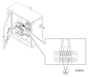
Figure 3-5. Remote Start Terminal Block
