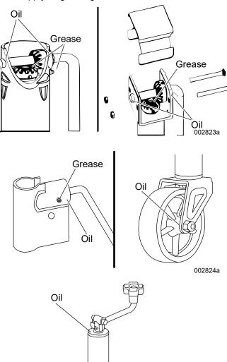
Figure 4-5. Lubrication Points
