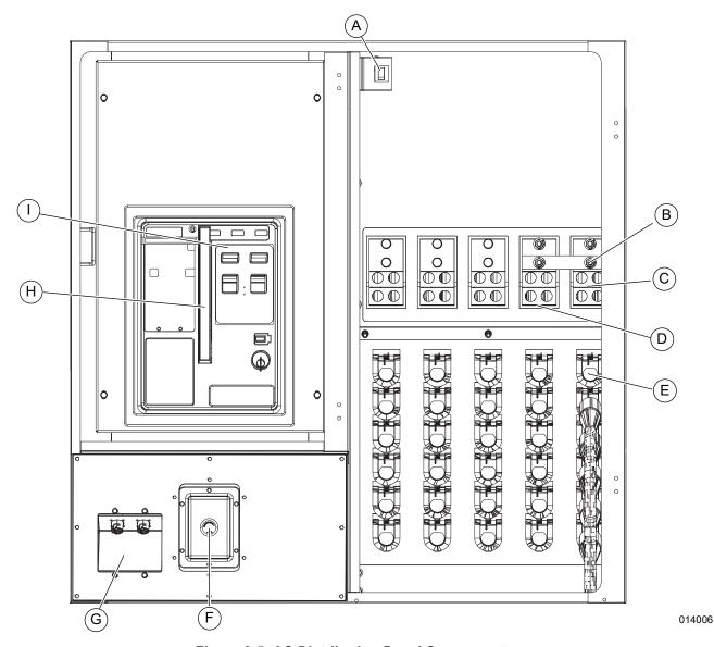
Figure 2-5. AC Distribution Panel Components
