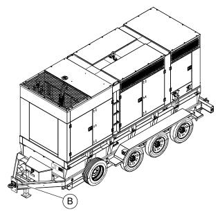
Figure 2-2. Unit ID and VIN Tag Locations
