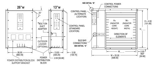
\*NOTE: IF DUCT ADAPTER IS USED, MOUNT USING LEFT & RIGHT FLANGES ONLY. OTHERWISE USE TOP AND BOTTOM FLANGES OF THE LOAD BANK.
