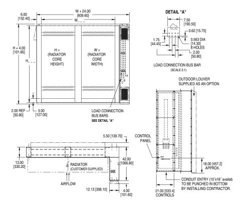
**NOTE:** Minimum core dimensions of 86" required for 1900 frame.
