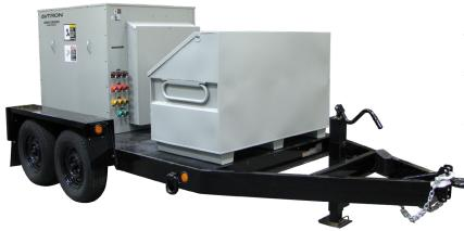
The Avtron Model 5500 are resistive, AC trailer mounted or trailer ready load banks designed for outdoor use when up to 500 kW of load is required.
