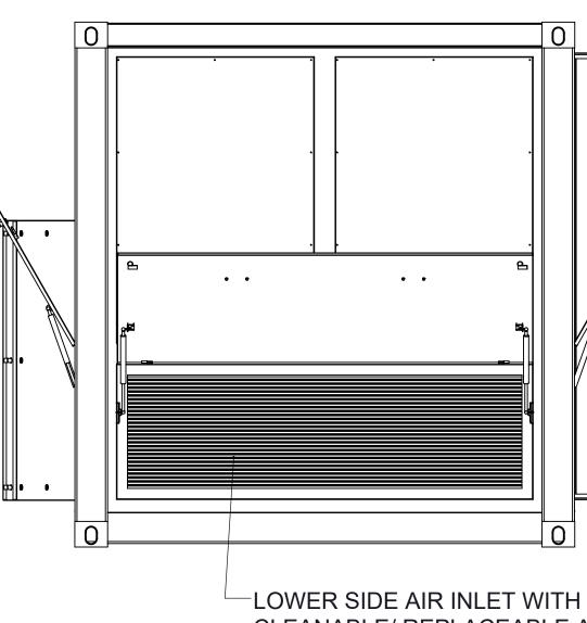
CLEANABLE/ REPLACEABLE AIR FILTER
