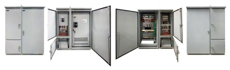
ASCO's SERIES 300 Manual Transfer Switch with Dual Purpose Quick Connects provide a reliable, convenient, and economical way to connect a both a standby generator and a Load Bank for testing. These units are available in models ranging from 150 to 3000 Amps. They are designed to provide years of trouble-free service. The switches are ETL listed to UL 891 Standards and provide an all-in-one solution for connecting temporary power during maintenance or repair of a permanent power source.
