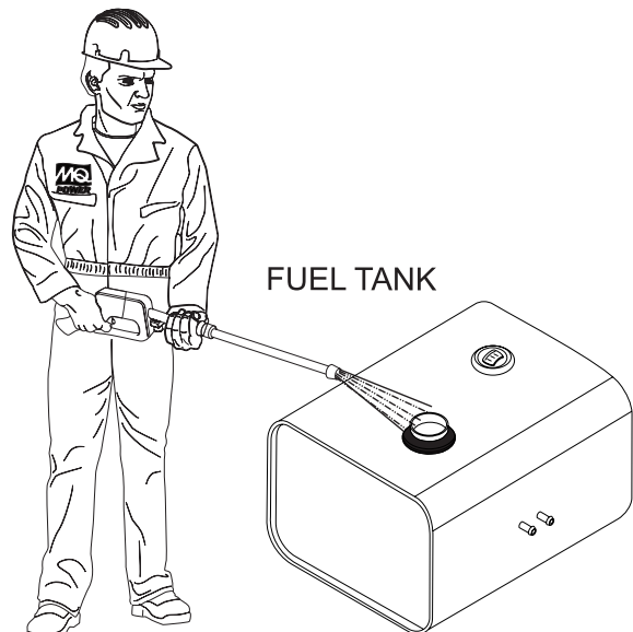
Figure 45. Fuel Tank Cleaning
