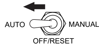
Figure 62. Auto Start/Stop Switch (Auto Position)
