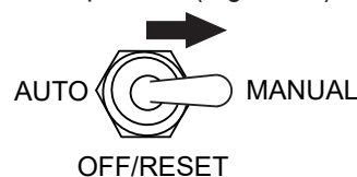
Figure 50. Auto Start/Stop Switch (Manual Position)
