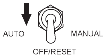
Figure 43. Auto Start/Stop Switch (Off/Reset)
