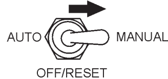
Figure 29. Auto Start/Stop Switch (Manual Position)
