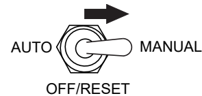
Figure 47. Auto Start/Stop Switch (Manual Position)
