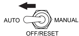
Figure 59. Auto Start/Stop Switch (Auto Position)
