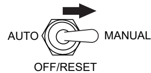
Figure 88. Auto Start/Stop Switch (Manual Position)
