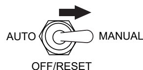
Figure 45. Auto Start/Stop Switch (Manual Position)
