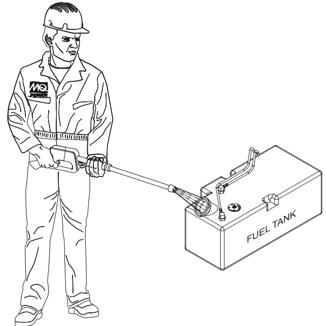
Figure 65. Fuel Tank Cleaning
