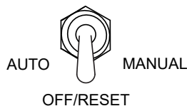
Figure 57. Auto Start/Stop Switch (Off/Reset)
