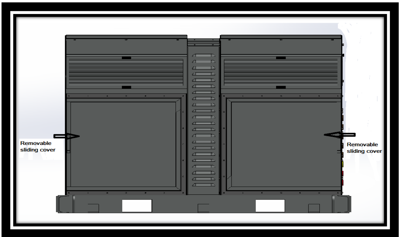
Figure-2 Sliding cover inlets
